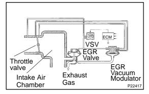
If even one of the following conditions is fulfilled, the VSV is turned ON by a signal from the ECM.
