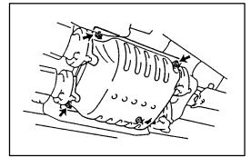
(g) Tighten the 2 bolts as shown in the illustration.
